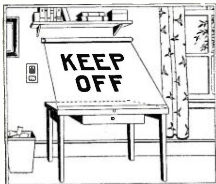
A window shade fixed in the position shown not only protects the table from dust but discourages the other members of the family from playing with your tools.
