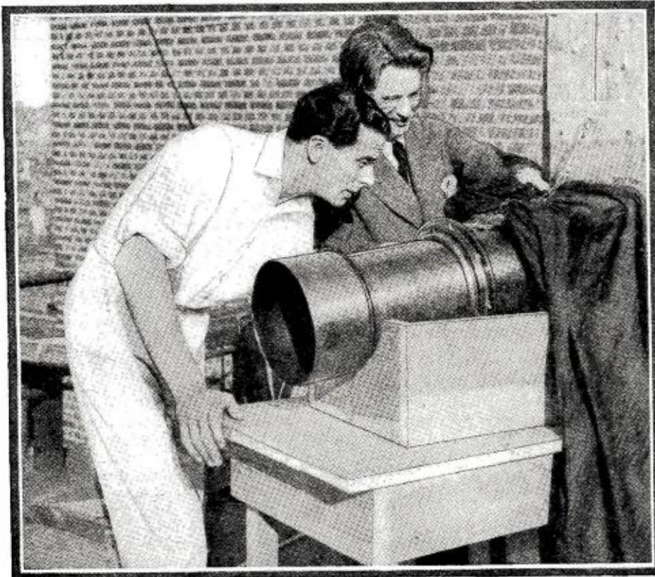
Mr. Baird (right) showing his television camera to an old schoolmate, Jack Buchanan, musical comedy star. Observe the light-gathering capacity of the lens, contained in the tube, behind which is the covered scanning mechanism.
