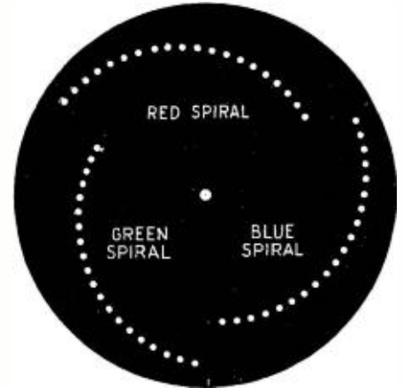
Arrangement of the spirals on the Baird multiple-colored television disc.
