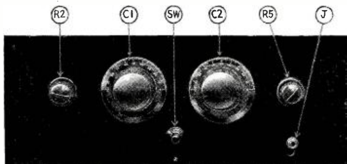
Fig. B. The two dials on the front panel of the "Milk-Shaker Special" receiver are the wavelength tuning controls. The knob R2 at the left is the volume control, and the knob R5 at the right is a regeneration control.
